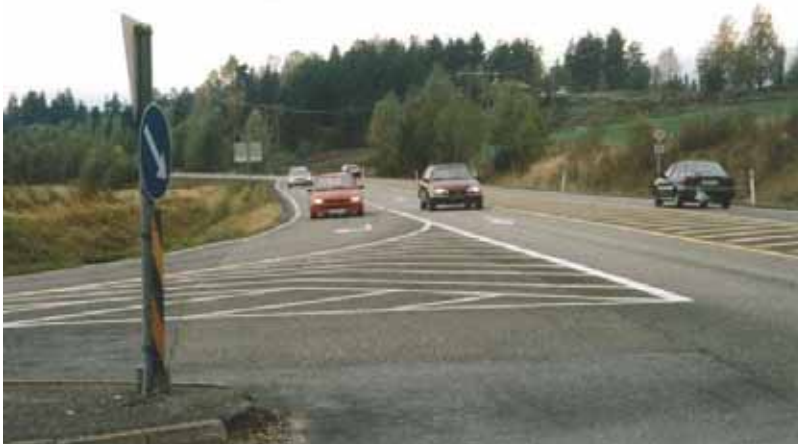
Figure 5.14 A large vehicle in the turning lane may hide a PTW in the through lane. (source: Norway Public Road Administration, MC Safety, Design and Operation of Roads and Traffic Systems, April 2004)
